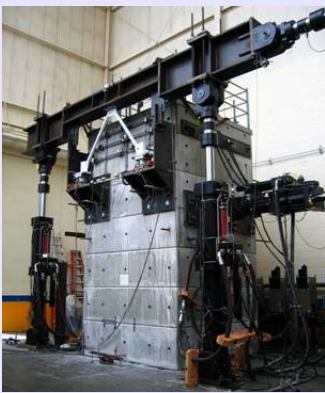
Hybrid test of the zipper frame
